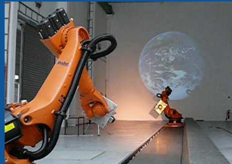
Final approach simulation with EPOS (GSOC DLR)
