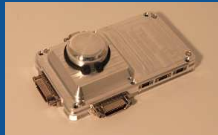
Assembled MCC-stack in casing with cabling and connectors
